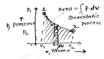
\* Work of expansion on the P-V diagram
